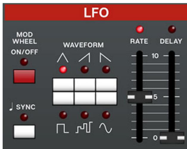
The low-frequency oscillator (LFO) generates sub-audio range signals intended for modulation purposes.
