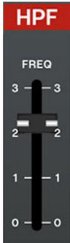
A highpass filter removes low frequencies as its cutoff frequency setting is increased, resulting in a thinning out of sound. The highpass filter section is a simple, non voltage-controlled affair, and acts more like a thickness control than a full-fledged filter.
