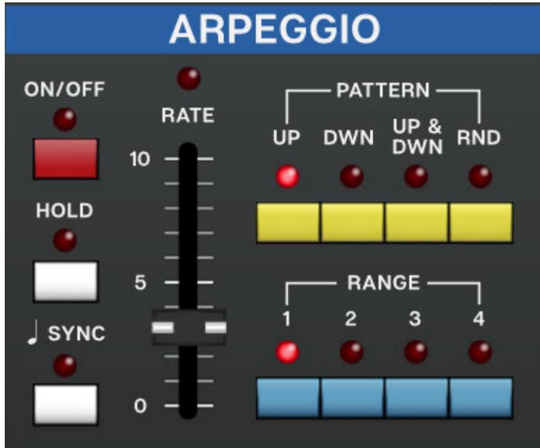
An arpeggiator is basically a step sequencer that plays each note of a chord individually in an ascending or descending pattern across one or more octaves. Though the original Juno-106 synth did not have any arpeggiator, the The DCO-106 *Arpeggio* section closely replicates the functionality of the Juno-6/Juno-60.
