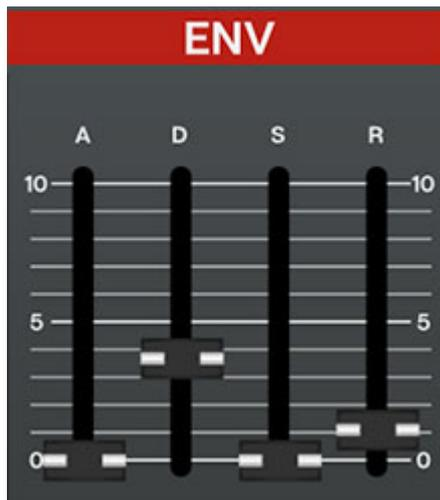
The envelope generator section is a standard ADSR envelope generator used to shape amplitude curves and/or filter CV. If you're not familiar with the operation of envelope generators, here's an overview:
