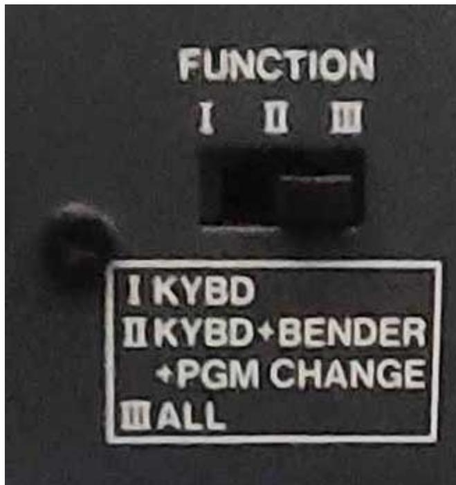
The *Function* switch on the Juno-106's back panel needs to be set to the *III* position for all this magic to work. Note that because it uses MIDI System Exclusive data, MIDI channel settings won't affect its operation (MIDI SysEx is not channelized and will not have unintended affects on other instruments or plug-ins.)
