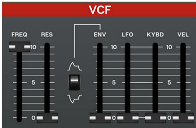
The VCF section is a 24 db/oct lowpass filter that removes high frequencies as its cutoff frequency setting is decreased from max, resulting in a dulling of sound. DCO-106 features a super-accurate emulation, with particular attention paid to the original Juno's non-linear self-resonating characteristics - phew, that's a mouthful, but all you gotta know is that DCO-106 sounds just like the real thing!
